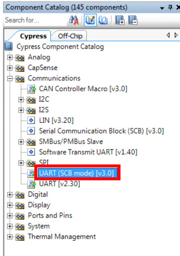
Figure 5-3. Open UART Configuration Window
