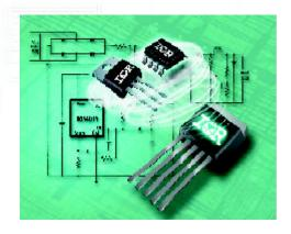
The IRIS Series integrated switchers combine a low-loss HEXFET® power MOSFET with a dual-mode voltage and current control IC and MOSFET gate drivers in a single 5-pin TO-220 or TO-262 package. The devices are optimized for flyback topologies in universal- and single-input, 30 to 180W switched mode power supplies (SMPS).
