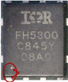
Figure 4 Pin 1 indicator on an IRFH5300PbF
