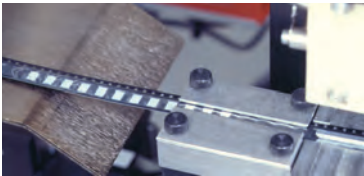
SureCHIP is packaged in tape after passing 100% electrical testing and visual inspection
